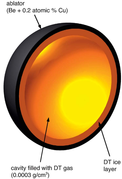
FIG. 5. (Color) Cross-sectional view of the base-line ICF capsule design developed by Vesey et al. [11,12]. The outer radius of the ablator R_c=2.65 mm, the outer radius of the DT-ice layer R_f=2.46 mm, and the inner radius of the ice is 2.18 mm. (This figure is a detail of the capsule illustrated in Fig. 1). Performance parameters for this capsule are listed in Table II.
